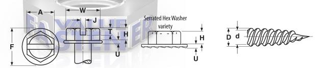
Head dimensions of self-piercing screws differ from those of standard tapping screws.
